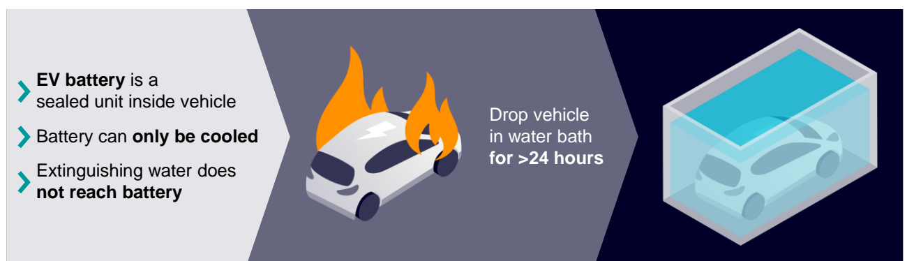
Figure 5: Water cooling of vehicles with battery fires
