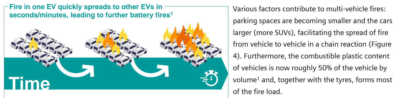
Figure 4: Fire quickly spreading from vehicle to vehicle
